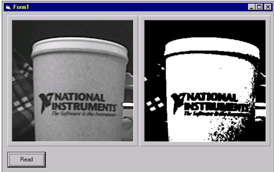
Figure 7-5. Testing the Image Acquisition Threshold Example
